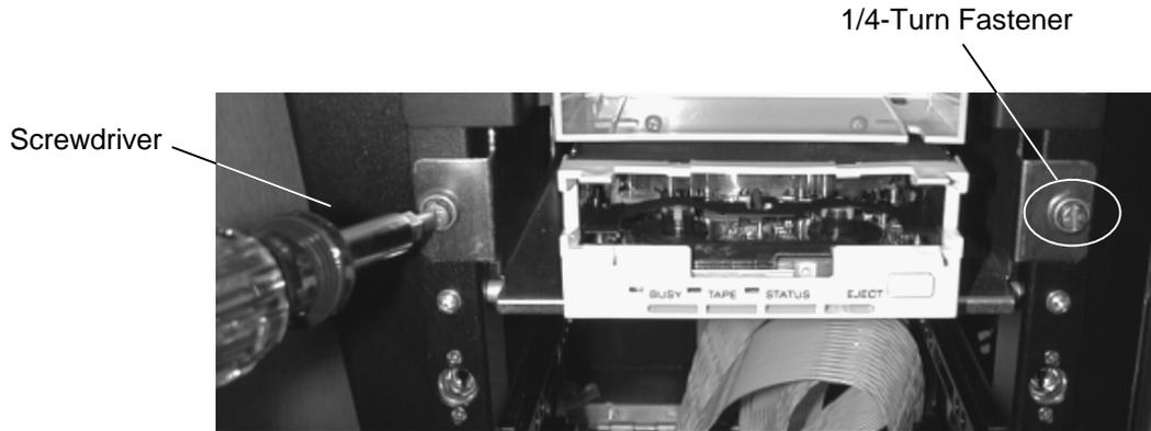
Figure 3-9 Installing the Drive into the Drive Bay
